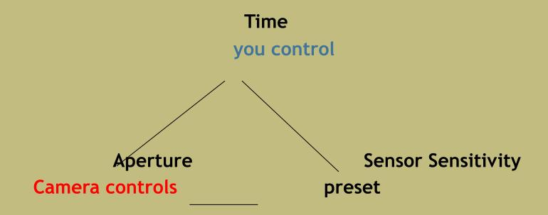
To maintain exposure the camera must change Aperture to compensate for the photographer's changes in shutter speed.
